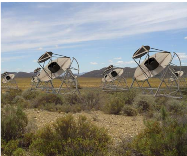
Fig 1. Left: Artist's vision of a possible layout of the proposed AGIS (Advanced Gamma-ray Imaging System; image courtesy of J.Buckley and V.Guarino). Right: One possible layout (with scale in meters) of the proposed CTA (Cherenkov Telescope Array) with 97 telescopes of which 3×4 have collecting areas of 600 m 2 each, and 85 others have 100 m 2 (figure by K.Berndlöhr 52 ).
