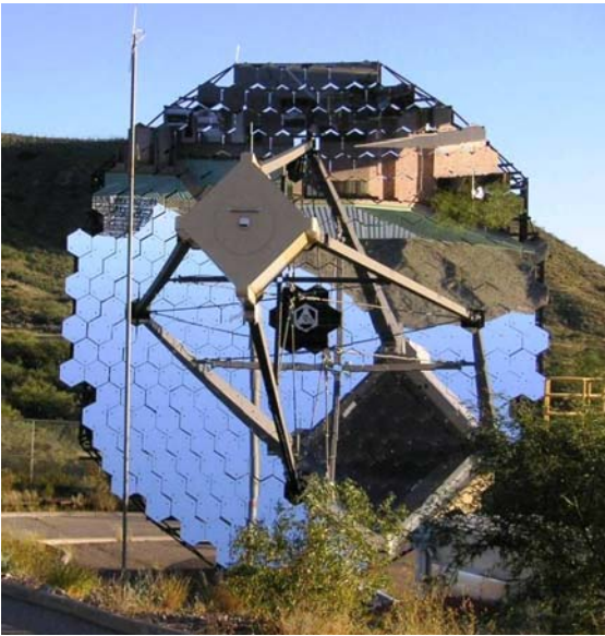
Fig. 4. Left: One of the four 12-m telescopes of the VERITAS array, used as a flux collector in the present experiments. The reflection of the photomultiplier matrix camera is seen. Right: Example of nanosecond-scale intensity cross correlations measured between one particular pair of VERITAS telescopes for the star 28 Cep (A2m; m_V = 5.8 ). The four curves illustrate how the signal converges as the integration times increase in the steps of 1-10-100-1000 seconds.
